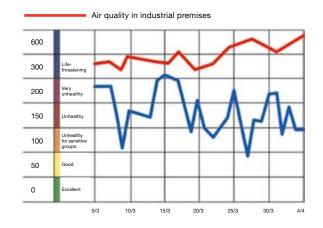
have entered the values for a standard manufacturing workplace where one of the main tasks is welding stainless steel. The measurements were taken to question background levels in the working environment. The graph clearly demonstrates that during the same 30-day period, air quality at the workplace was considerably worse than the air quality in Beijing.
